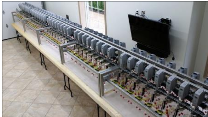
Rare Earth Solvent Extraction Pilot Plant
