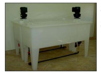
Project: sxk-141 Client: Rio Tinto Australia Location: Australia Stages: 2 Capacity: 26 L/min (org + aq) Recycle: optional organic or aqueous
