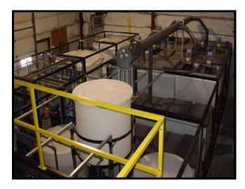
Project: sxk-37 Client: Moscow State Institute of Steel and Alloys (Technological University) Location: Moscow, Russia Stages: 4 Capacity: 100 L/min (org + Aq) Recycle: optional organic or aqueous
