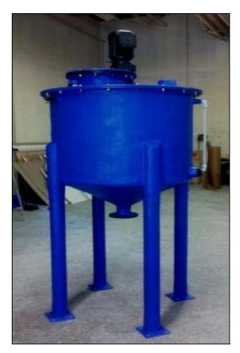
Item: Agitation Leach Tank Project: sxk-156 Client: Royal Canadian Mint Capacity: 500 L Stages: 1 Temperature: 20 to 80 °C Drive: 1 Hp inline gear motor with VFD
