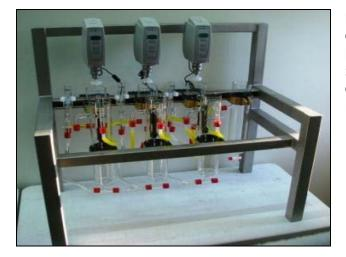
Project: sxk-158 Client: Equilab Chile Location: Chile Stages: 3 Capacity: 150 mL/min (org + Aq) Recycle: Option for organic or aqueous
