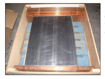
Item: Anodes Project: sxk-38 Client: Moscow State Institute of Steel and Alloys (Technological University) Location: Moscow, Russia Quantity: 60 Dimensions: 800 mm x 700 mm
