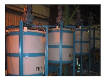
Item: CCD Circuit Project: sxk-20 Client: MRSI / CMS / Cotter Corp Location: Canon City, CO, USA Capacity: 10 L/min of feed slurry Stages: 4 Temperature: 20 to 60 °C Drive: fixed speed
