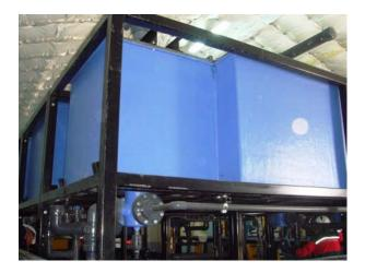
Project: sxk-105 Client: Shepherd Chemical Location: Norwood, OH, USA Stages: 9 Capacity: 30 L/min (org + aq) Recycle: optional organic or aqueous
