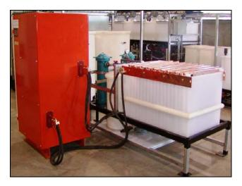
Project: sxk-55 Client: IMPRC Location: Tehran, Iran Capacity: 1,250 g Copper per hour Cathodes: 8 Anodes: 9 Rectifier: 0 to 1000 amps, 0 to 4 volts
