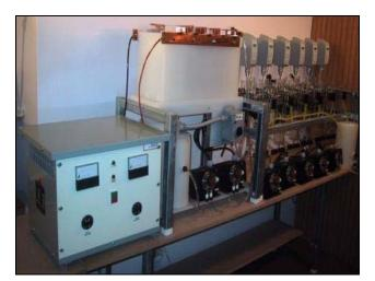
Project: sxk-44 Client: Erdenet Mining Corporation Location: Erdenet, Mongolia Capacity: 60 g Copper per hour Cathodes: 4 Anodes: 5 Rectifier: 0 to 50 amps, 0 to 5 volts
