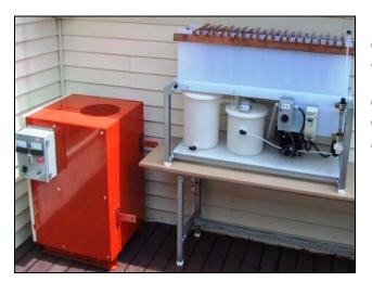
Project: sxk-41 Client: Southern Peru Copper Corporation Location: Toquepala, Peru Capacity: 208 g Copper per hour Cathodes: 10 Anodes: 11 Rectifier: 0 to 300 amps, 0 to 5 volts
