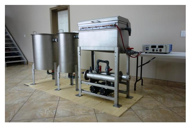
Gold EW plant manufactured from stainless steel for operation at high temperature.
