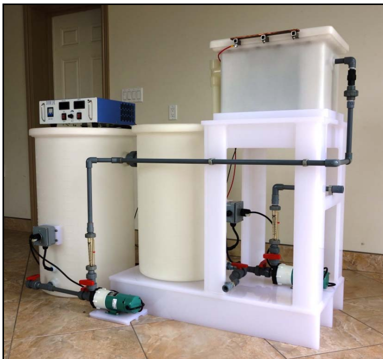
Gold EW plant with 50 A rectifier
