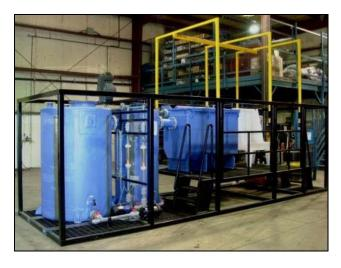
Project: sxk-142 Client: Soltin Investments Inc. Location: Cuba Capacity: 100 kg gold per week Cathodes: 9 Anodes: 10 Rectifier: 0 to 450 A and 0 to 4 V
