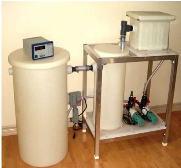
Gold EW pilot plant with 5 A rectifier
