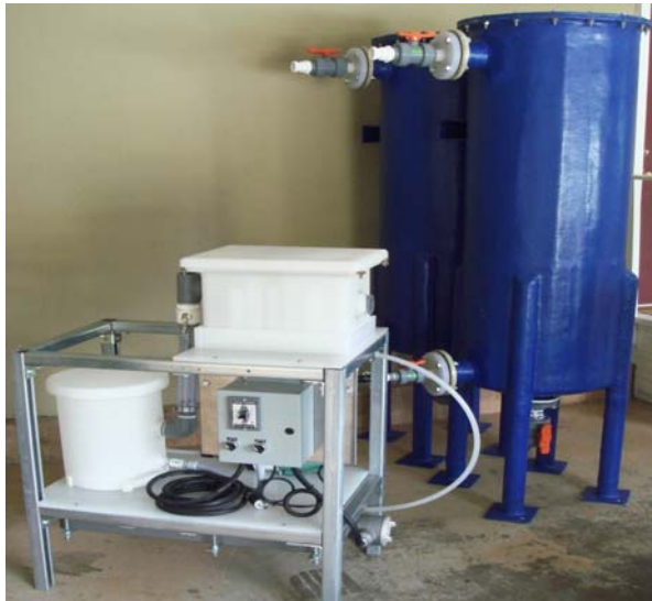
Gold EW pilot plant with carbon columns
