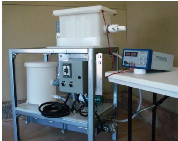
Gold EW pilot plant with 5 A rectifier
