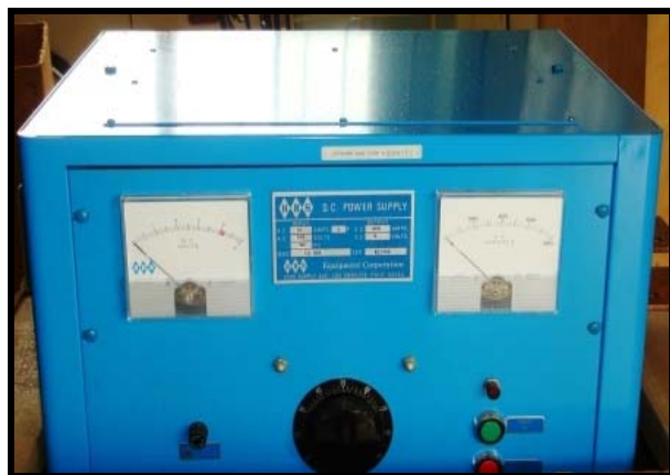
0 to 800 A and 0 to 4 V rectifier
