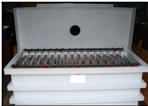
EW cell with 15 cathode boxes and 16 anodes
