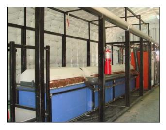
Project: sxk-76 Client: Sary Kazna LLP Location: Balkhash, Kazakhstan Capacity: 240 kg copper per day Cathodes: 40 Anodes: 55 Rectifier: 0 to 2,500 A and 0 to 12 V
