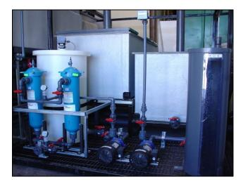
Item: Continuous Coalescer Project: sxk-37 Client: Moscow State Institute of Steel and Alloys (Technological University) Location: Moscow, Russia Capacity: 50 L/min aqueous flow
